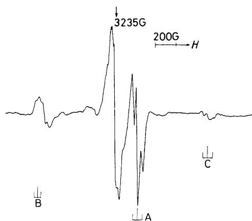
Figure 4. First-derivative X-band e.s.r. spectrum for a dilute solution of \text{Hg}(\text{C}_2\text{H}_5)_2 in \text{CFCl}_3 , showing the perpendicular feature assigned to \text{Hg}(\text{C}_2\text{H}_5)_2^{*+} cations, with a triplet splitting of 42 G assigned to hyperfine coupling to two equivalent protons. The extra central line is due to organic radicals
